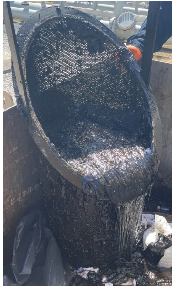
Figure 1: 12" Facility Strainer Plugged with Sludge
